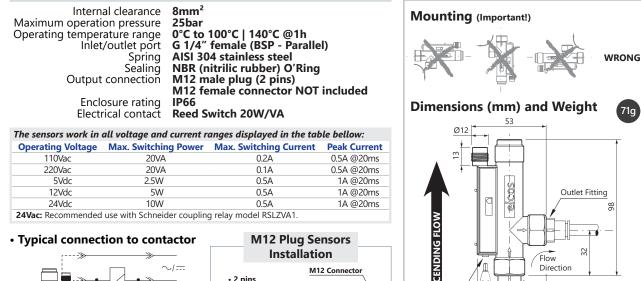
• 2 pins **A**-codina {**K8** for AC **KD** for DC Snubber Filter F Installing the snubber filter extends the lifespan Flow Switch of the sensor's electrical contact.
